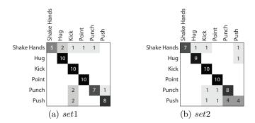
**Fig. 2.** Confusion matrix for classification of group actions for (a) set 1 and (b) set 2 using the min rule for classifier fusion.
